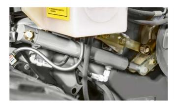
Blockages in the intake can be cleared quickly and easily by reversing the rotor mechanically using the rotor lever. The optionally available hydraulic rotor unblocking unit can be activated from the cab and allows the baler to be driven right up to its performance limits without any problems.
