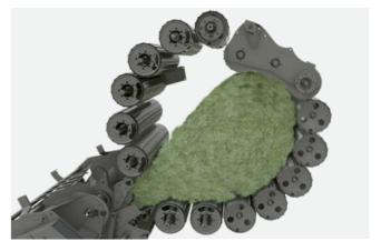
Hydraulic MAXIMUM PRESSURE PLUS for the ROLLANT 455 and ROLLANT 455 UNIWRAP.
