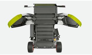
The 17 HD rollers, with a significantly thicker casing, process the crop into firm 1.22 x 1.50-m bales with excellent shape retention – with net wrapping or twine tying as desired.
