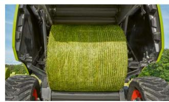
The ROLLANT 540 opens and closes the tailgate automatically in just six seconds once the operator puts the tractor in neutral. The operator's workload is further reduced by the automatic knife cleaning cycle, automatic knife deactivation and convenient knife group activation from the cab.
