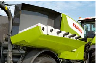
table, which is tilted towards the bale chamber, where the bale is guided along by an array of large rollers.
