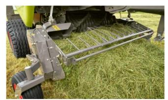
The controlled pick-up adjusts to any ground contours, even at high working speeds and while negotiating curves. Large guide wheels with tool-free adjustment keep you safely on track at all times.
