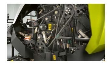
All drives are straight and mounted completely on the lefthand side. This allows the power to be transmitted with optimum efficiency. In the ROLLANT 540, only large long-life Tsubaki chains are used, which are lubricated with a constant oil film.
