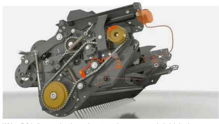
With a 7.2-I oil reservoir volume, the automatic, permanent chain lubrication ensures reliable operation on long working days and a long service life. The oil quantity can be adjusted independently of the operating conditions.
