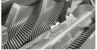
Knife group activation allows you to react flexibly to the requirements of the job at hand. The knife groups can be preselected on the machine and extended or retracted via the control terminal.
