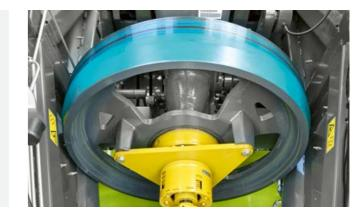
The new flywheel version: increased mass and inertia for improved impact.
