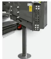
The hydraulic jack makes it quick and easy to attach the baler.
