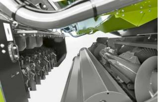
The double spiral rotor with 88 knives ensures high cutting quality and even crop flow at a working width of 2 metres. The two rows of knives can be set up as shear bars at several levels with 45 knives each.
