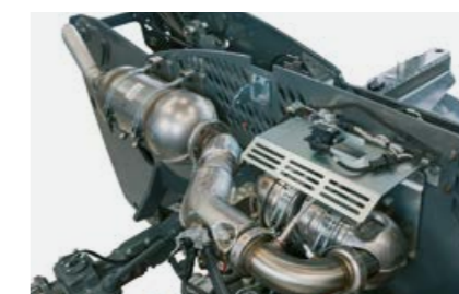
The diesel particulate filter is regenerated automatically.
