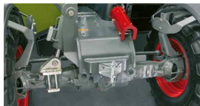
Greater off-road safety thanks to hydraulic levelling
