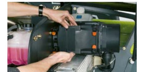
Sockets for a flexible power supply to a wide range of attached and trailed implements
