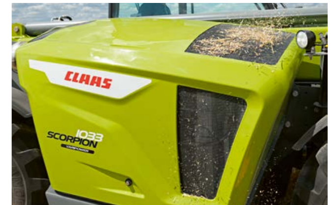
Avoidance of radiator soiling thanks to the reversible fan
