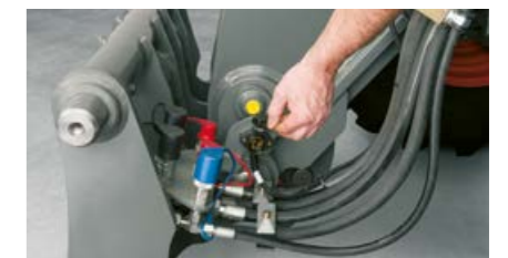
Sockets for a flexible power supply to a wide range of attached and trailed implements
