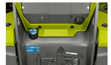
Easily accessible AdBlue®-filler neck filler neck for efficient exhaust gas aftertreatment
