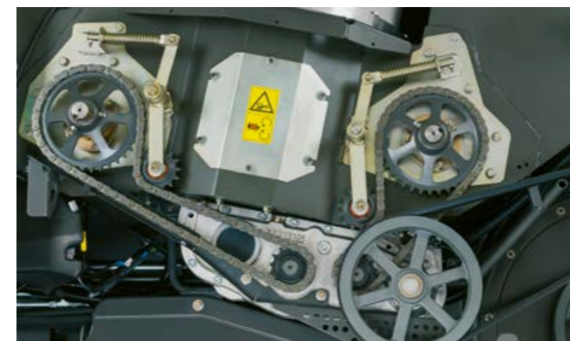
180 l/s unloading drive system
