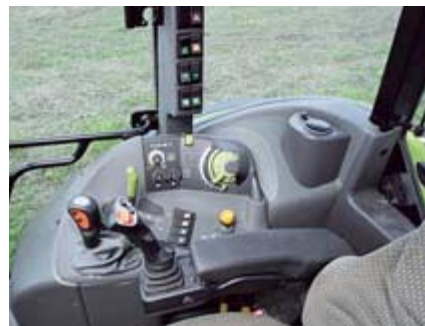
Optional ElectroPilot joystick on the armrest operates two spool valves and the powershift splits, while the controls on the hand throttle lever also shift through transmission ranges.
