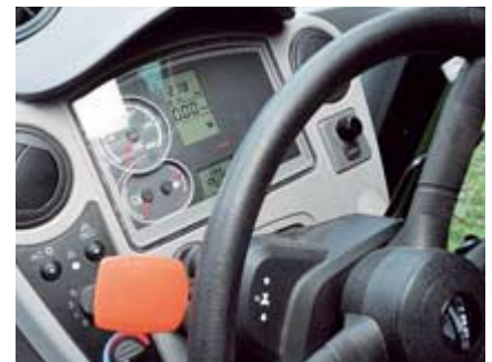
The dash presents a vast array of information, but the display at the bottom could do with being larger. The dial/button on the right allows the operator to scroll through settings.
