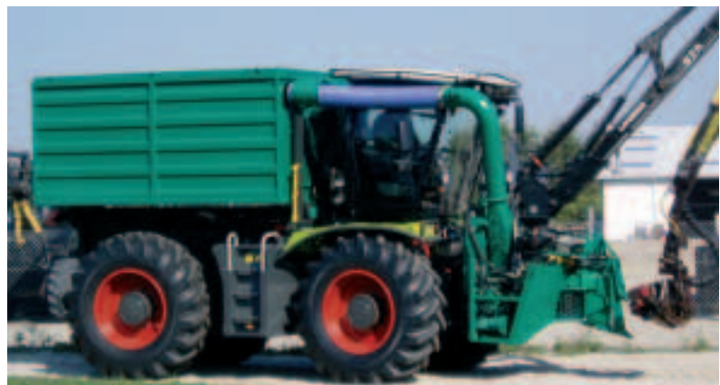
The XERION with a fixed woodchipper, grabber crane and 18 m 3 bunker.
